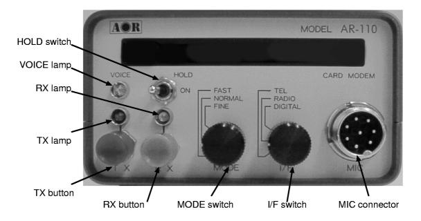
TX switch button --- Push to transmit RX switch button --- Push to force receiving or transmit send request TX LED lamp ----- Lit while transmit RX LED lamp ----- Lit while in the receive standby mode VOICE LED lamp -- Voice communication is available when lit MIC connector -- Connect a radio microphone PC card slot ----- Insert a PC card HOLD switch --- Switch to HOLD side to disable receiving I/F switch ------ Select an interface mode MODE switch -- Select a picture quality
